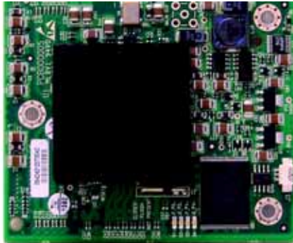
Figure B-2. AOC-IBH-002 Mezzanine HCA Card
