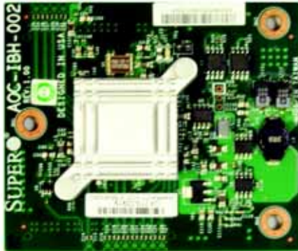
Figure B-2. AOC-IBH-002 Mezzanine HCA Card
