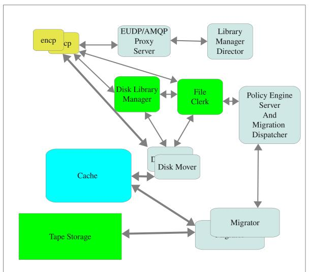
Fig 1. Structure of integrated data caching and tape system using encp and disk movers.
